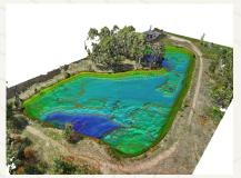
Our bathymetric surveys are conducted using high-precision unmanned surface vehicles (USVs) equipped with singlebeam echo sounder, delivering accurate underwater terrain data in lakes, rivers, ponds, and tailings.
