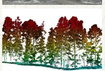
We use high-end LiDAR sensors and high-resolution aerial cameras to deliver industry-leading mapping precision. Our UAV-mounted LiDAR systems support up to 16 returns per pulse, enabling exceptional vegetation penetration and highly accurate bare-earth modelling, even in dense forested environments.
